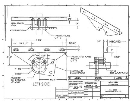
Blueprint of wheel pant fairing bracket (axel plug on next page)
