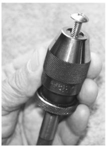
Screw held in chuck for sharpening
