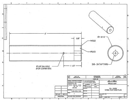
Blueprint of wheel pant fairing hardware --- axel plug
