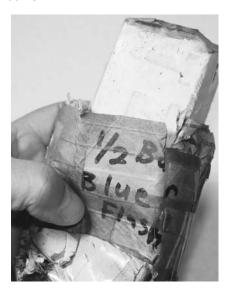
out from a man in the plating/polishing business that the ultimate deep, transparent shine is achieved by the application of a "Blue Flash" polishing bar. The results of this product are spectacular. Some people use buffing products that are liquid which when applied to a wheel rotating at 3500RPM . . . . WOW! Not safe city.
